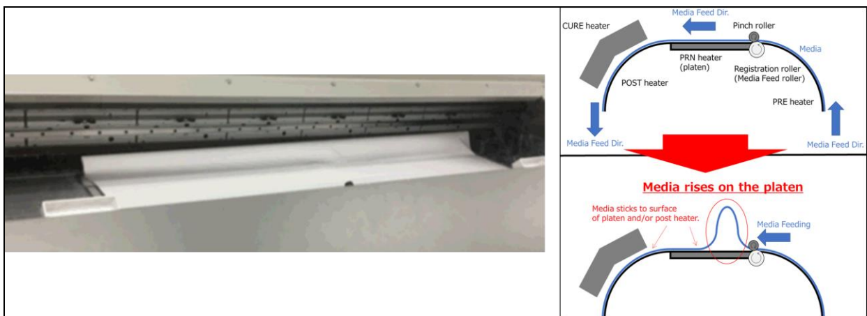
Fig. Photo and schematic illustration of risen media on the platen.
