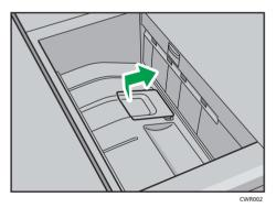
When you have finished using the Z-fold support tray for multi-folding unit, lift it up and slide the tray to the left, and then lower it.
