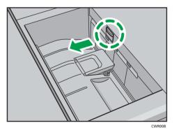
When you have finished using the Z-fold support tray for multi-folding unit and the output holding unit for letter fold-out, return each to their previous positions.
