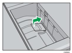
2. Pull out the output holding unit for letter fold-out.
