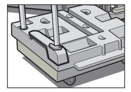
Be careful to push the stacker cart in straight, not at an angle.
