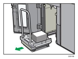
4. Rest the paper press on top of the paper stack.
