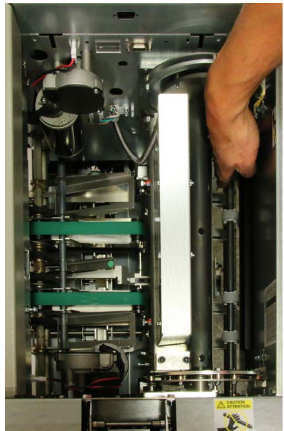
infeed roller shaft assy. lifted
