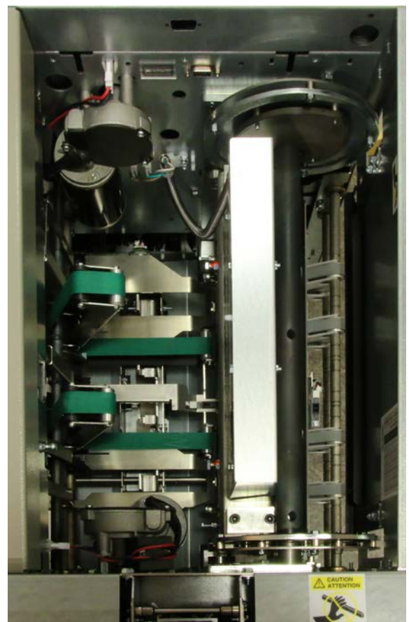
Exit compressing brackets lifted
